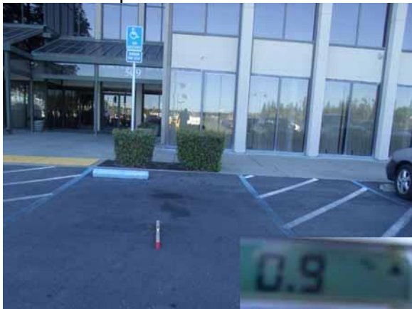
This section of slope is compliant
