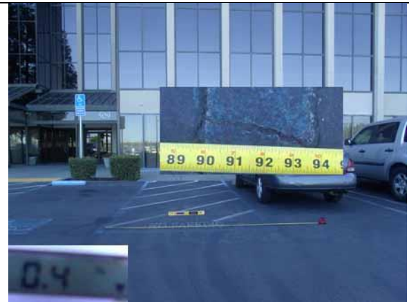
Van Access aisle shall be 8' wide minimum
