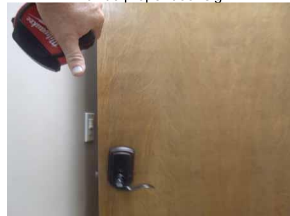
This door operation forces exceed allowable
